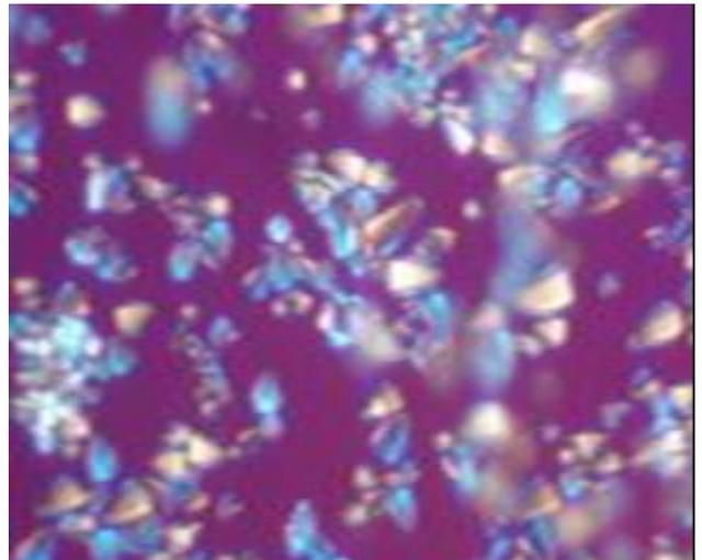
**Fig. 1.** Micrograph of the *Dioscorea bulbifera* starch granules using optic microscopy (OPM) 10x
